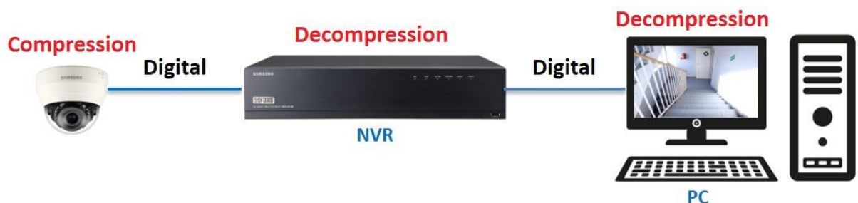
Figure (3-3): IP-Based CCTV System
