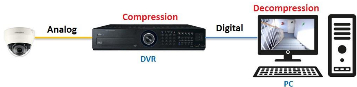
Figure (3-2): Analog CCTV System
